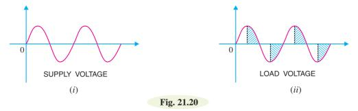
The firing of triac can be controlled upto a maximum of 180°. In this way, we can provide a continuous control of load voltage from practically zero to full *r.m.s.* value.
