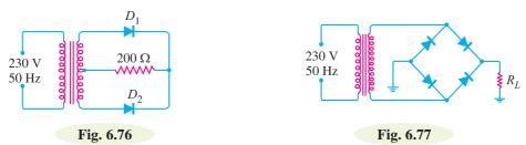
7. In Fig. 6.76, the maximum voltage across half of secondary winding is 50 V. Find (i) the average load voltage (ii) peak inverse voltage (iii) output frequency. Assume the diodes to be ideal.
