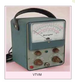
Range selection. In practice, a *VTVM* is made a multirange instrument by employing a potentiometer at the input circuit as shown in Fig. 22.13. By throwing the range selector switch *S* to a suitable position, the desired voltage range can be obtained. Thus when the range selector switch *S* is thrown to position 1, the voltage applied to the grid is three times as compared to position 3. Although only three voltage ranges have been considered, a commercial *VTVM* may have more ranges.
