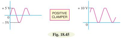
A clamping circuit (or a clamper) essentially adds a d.c. component to the signal. Fig. 18.45 shows the key idea behind clamping. The input signal is a sine wave having a peak-to-peak value of 10 V. The clamper adds the d.c. component and pushes the signal upwards so that the negative peaks fall on the zero level. As you can see, the waveform now has peak values of +10 V and 0 V.
